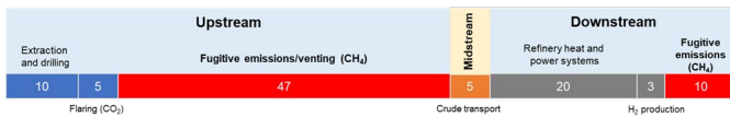
Figure 2: Types of emissions in the oil and gas value chain, by source and share
